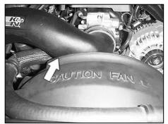
13. Due to production tolerances it may be necessary to mark the fan shroud as indicated, remove the intake tube and trim the fan shroud. **NOTE: Be sure to cover the throttle body and alternator during this process.**
