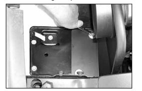
14. Adjust the heat shield and intake tube for best fit, then tighten the two hex bolts as shown.
