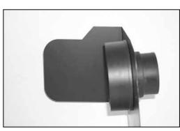
7. Assemble the mass air adapter, heat shield, gaskets and the mass air sensor as shown above.
