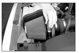
15. Install the K&N<sup>®</sup> air filter onto the heat shield assembly as shown.
