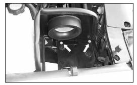
9. Install and mount the heat shield assembly to the air cleaner mounting tray using the bolts removed in step 5.
