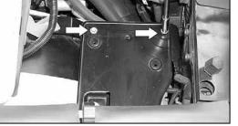
5. Loosen and remove the two air cleaner mounting tray bolts as shown.
